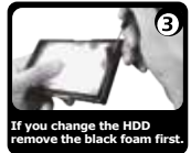
Insert the black foam in the gap between HDD and frame if necessary.
