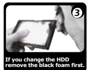
Insert the black foam in the gap between HDD and frame if necessary.
