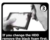
Insert the black foam in the gap between HDD and frame if necessary.
