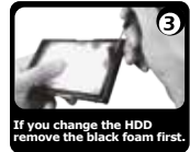
Insert the black foam in the gap between HDD and frame if necessary.
